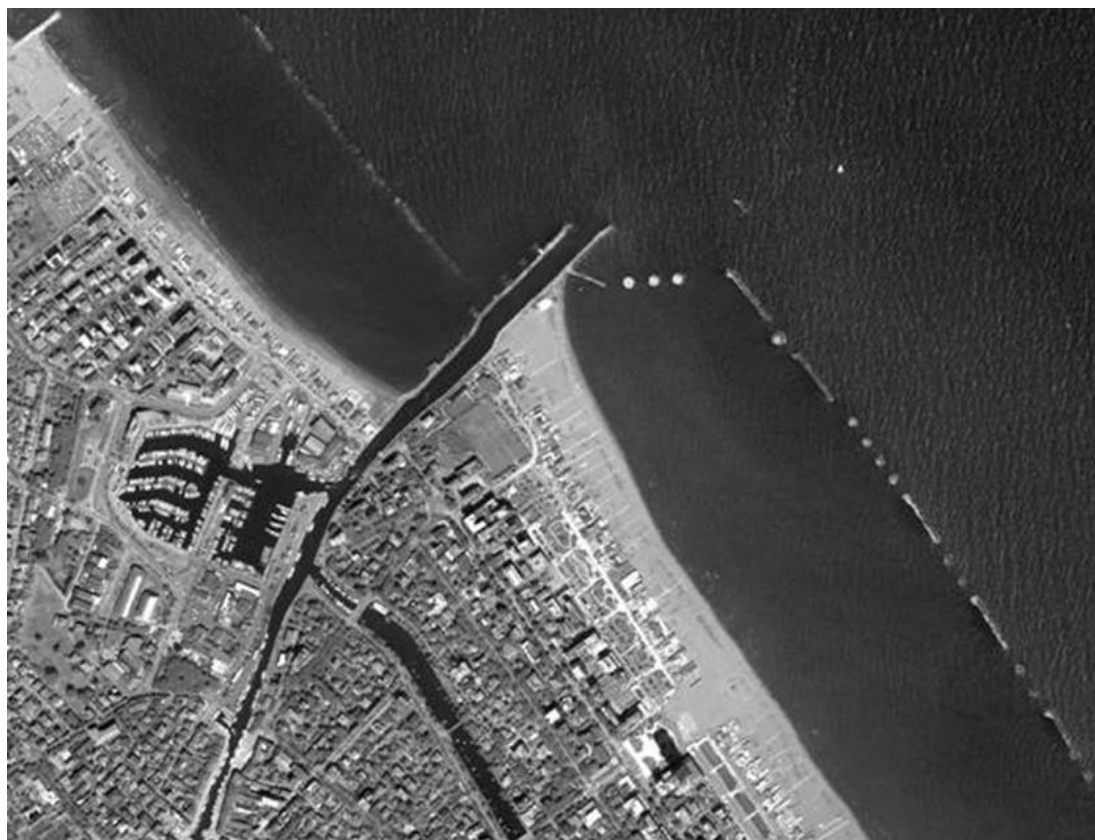
Figure 4 - Asymmetry of the coastline due to the sediment belt interruption imposed by the Cesenatico pier; the overflow side is accreting while the underflow side lacks sedimentation (Perini et al. , 2008).
